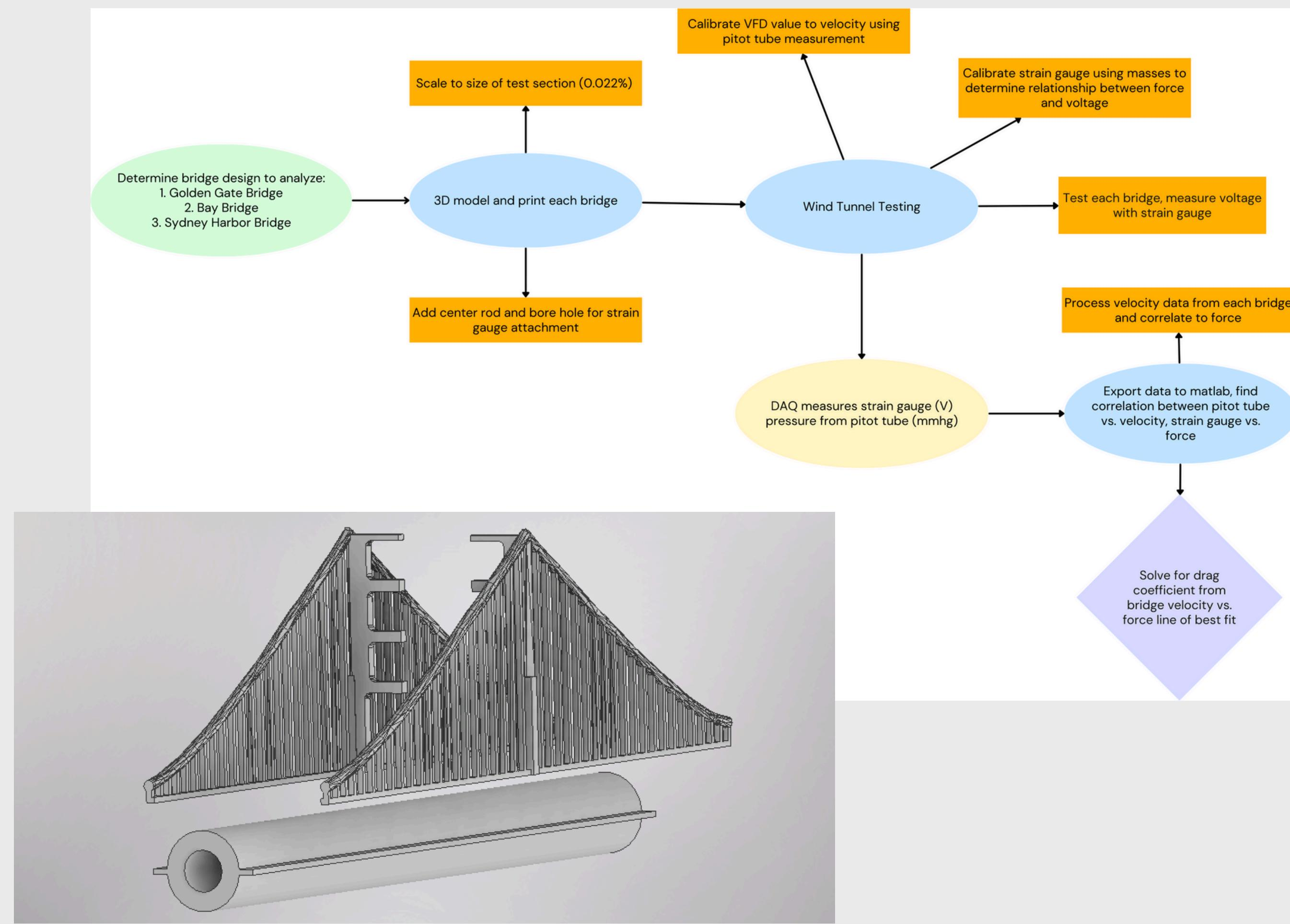
The design of our procedure revolved around the usage of the wind tunnel, specifically defining a max test section area of 6 in<sup>2</sup>. Our bridge models optimized this required area with reference to the strain gauge in order to measure aerodynamic response to varying wind velocities. The bridges proved difficult to re-create in one piece on 3D printers. As a result, each bridge was printed as a composite and pieced together after printing.
